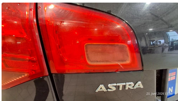
2.2 Krakelering i plast
