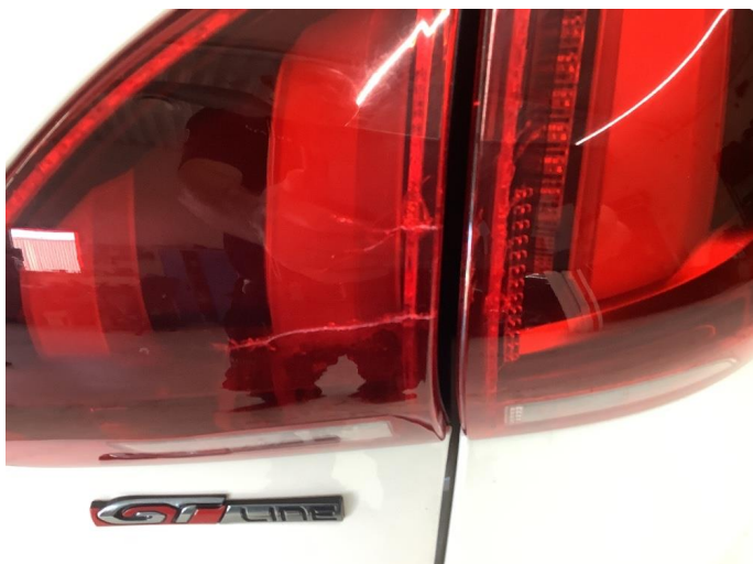
1.1 Krakelering i plast
