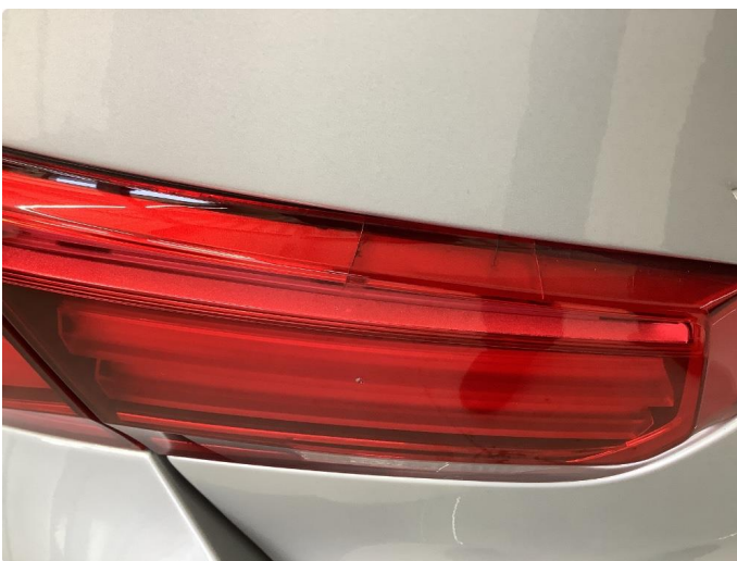
2.1 Krakelering i plast
