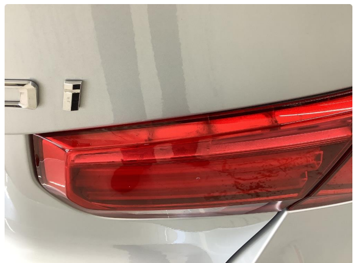
2.1 Krakelering i plast
