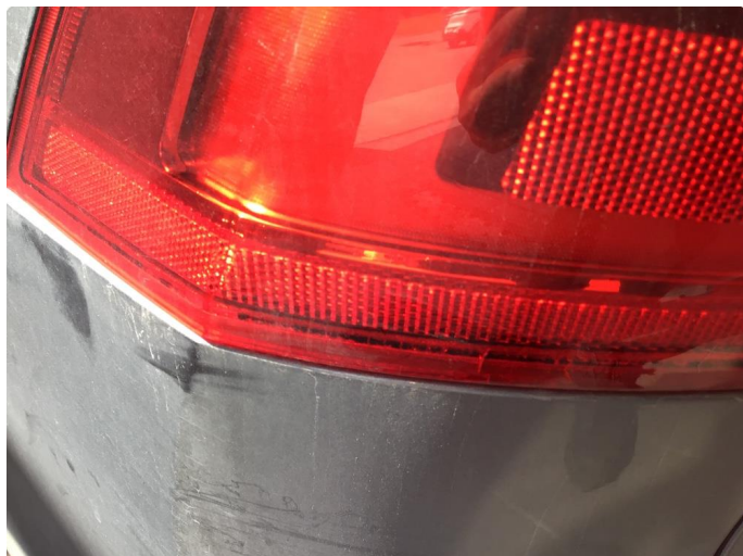
2.1 Krakelering i plast
