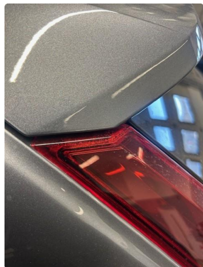
2.1 Krakelering i plast
