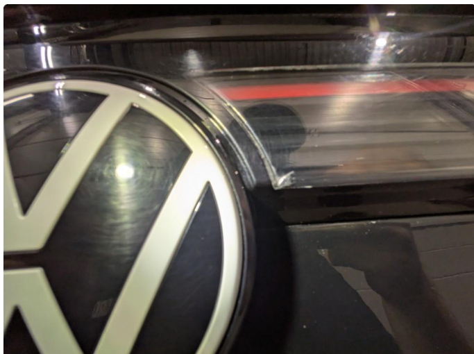
1.1 Krakelering i plast
