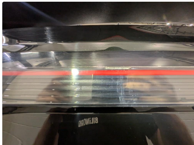
1.1 Krakelering i plast
