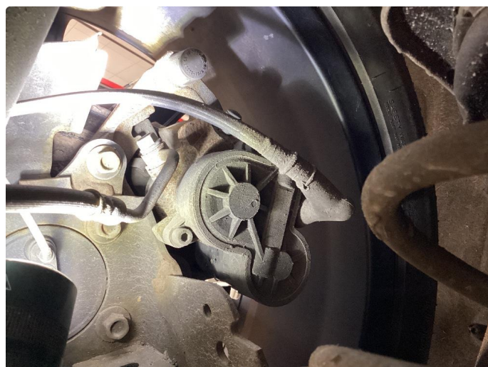
2.1 Mer enn 25% rust
