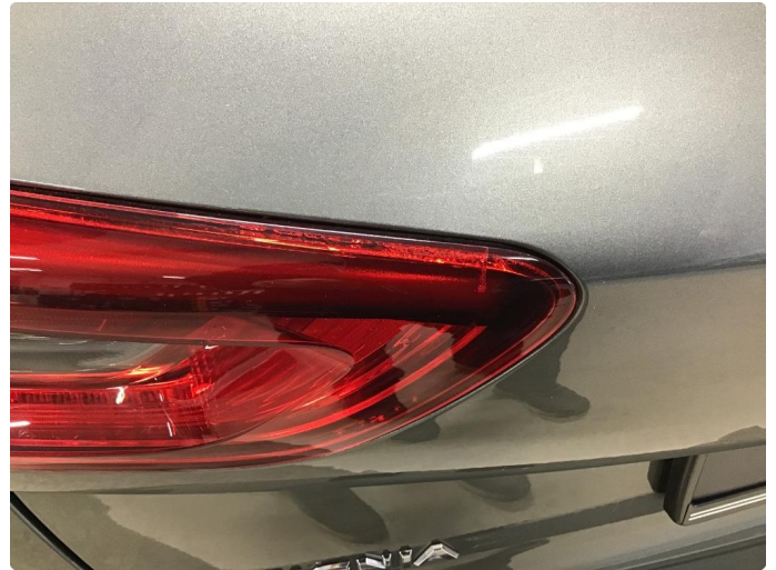
2.1 Krakelering i plast
