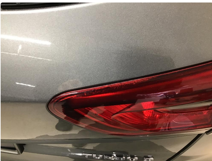
2.1 Krakelering i plast
