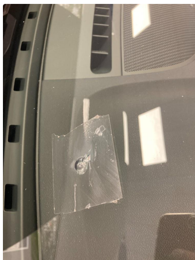
1.2 Steinsprut i synsfelt
