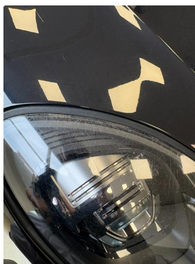
2.1 Krakelering i plast
