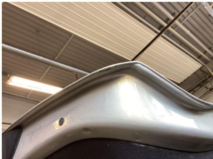
1.2 Rust i fals
