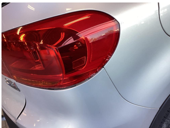
2.1 Krakelering i plast
