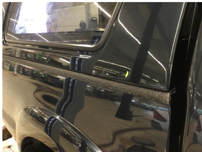
1.1 Sprekk i gailcoat h.side plantopp.
