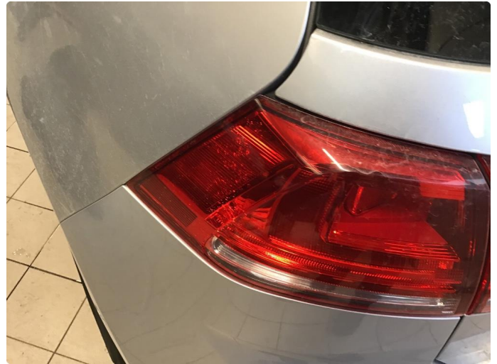
2.1 Krakelering i plast
