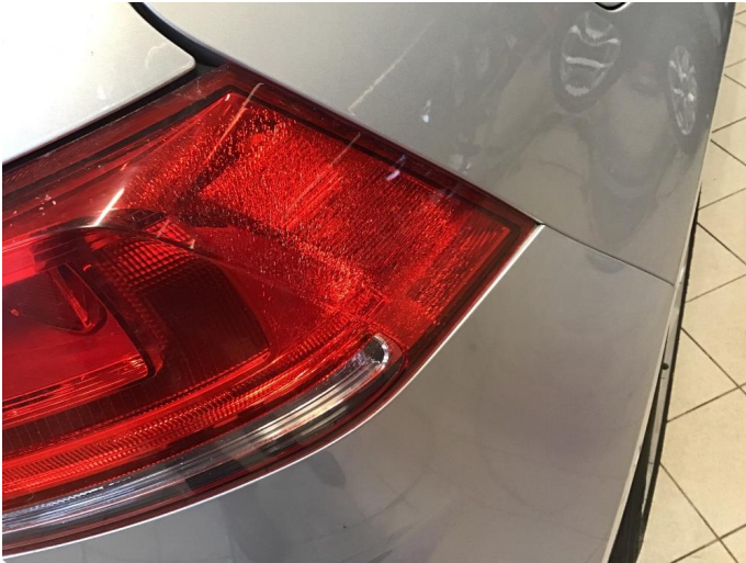
2.1 Krakelering i plast
