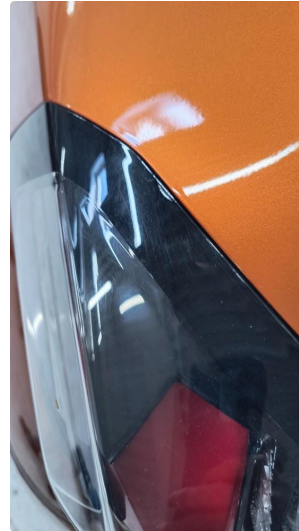
1.2 Krakelering i plast
