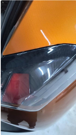
1.1 Krakelering i plast
