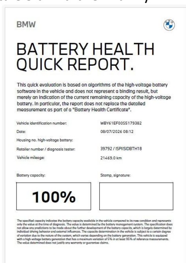
3.1 Test HV-Battery Condition OK, 100 %
