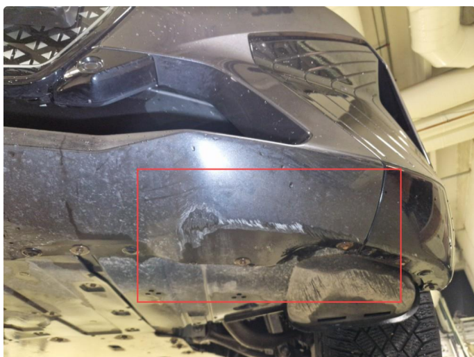
1.2 Skrubbskader underside frontfanger .
