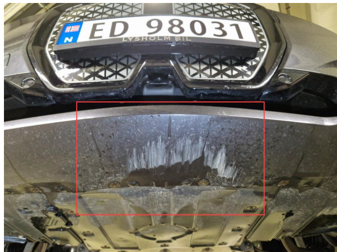
1.2 Skrubbskader underside frontfanger .
