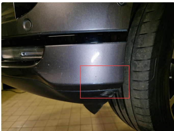
1.7 Lakkskader v-side frontfanger.
