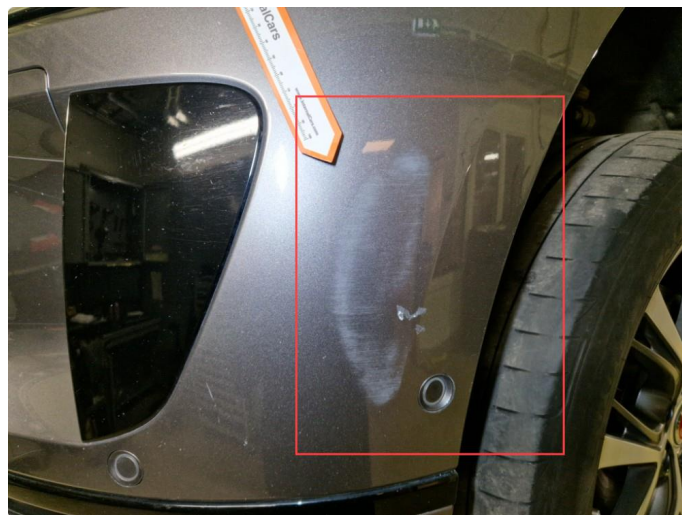
1.7 Lakkskader v-side frontfanger.
