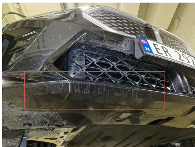
2.3 Noen skrubbermerker underkant fremfanger.
