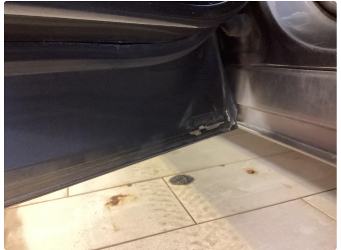
1.2 Rust i fals
