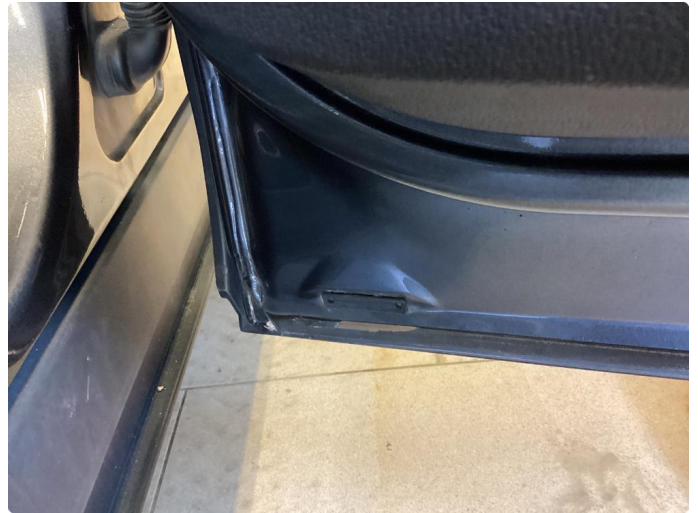
1.2 Rust i fals
