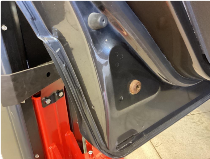
1.2 Rust i fals
