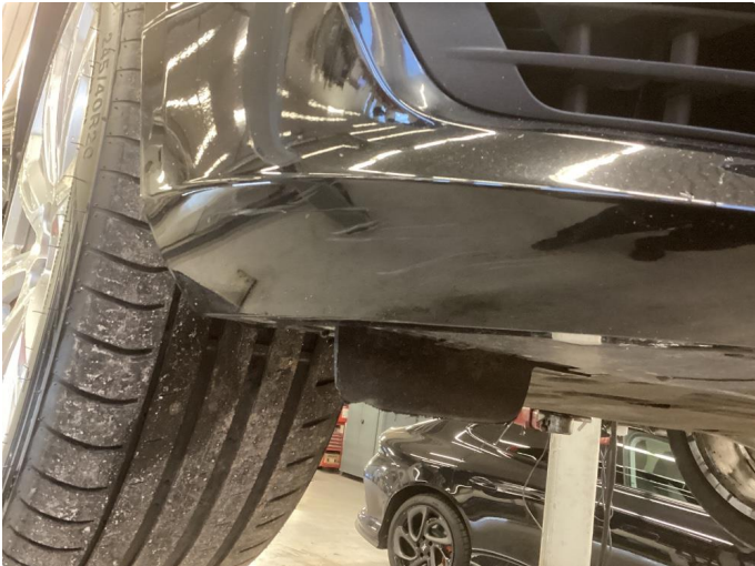
1.2 Liten skade under fanger
