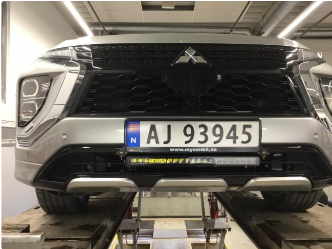
1.1 Ledbar montert under skilt.
