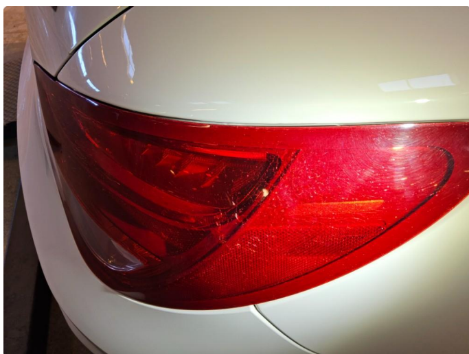
2.1 Krakelering i plast
