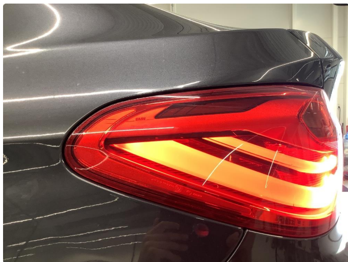
2.2 Krakelering i plast
