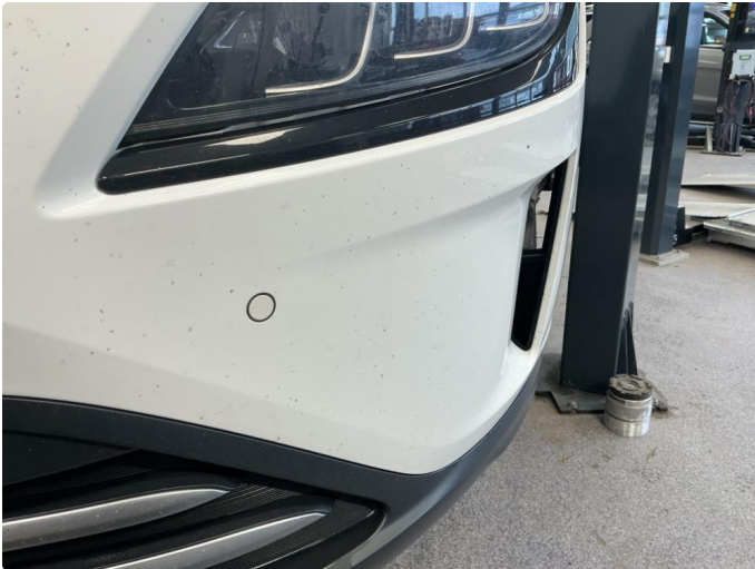
1.1 Noe steinsprut i frontfanger
