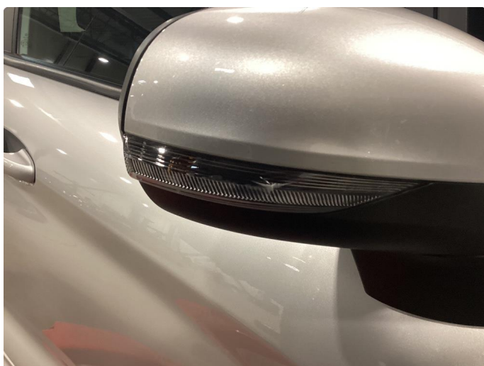
2.1 Krakelering i plast
