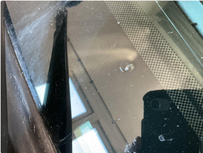
1.1 Steinsprut utenfor synsfelt
