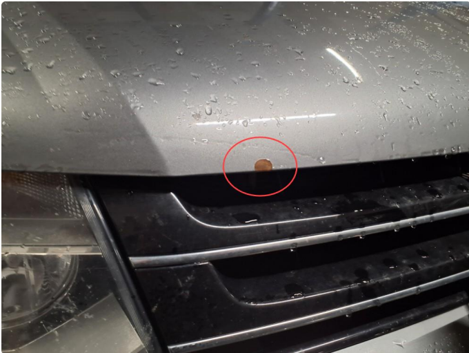
1.2 Rust i fals
