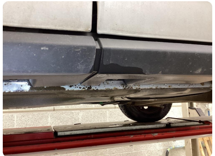
1.2 Rust Anbefaler rust behandling under
