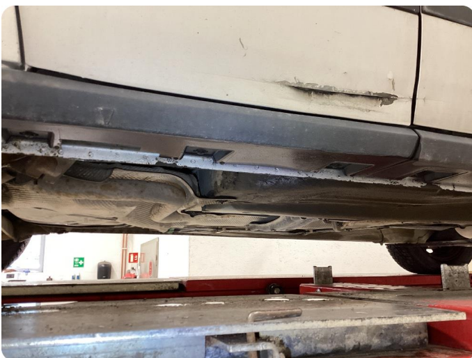
1.2 Rust Anbefaler rust behandling under
