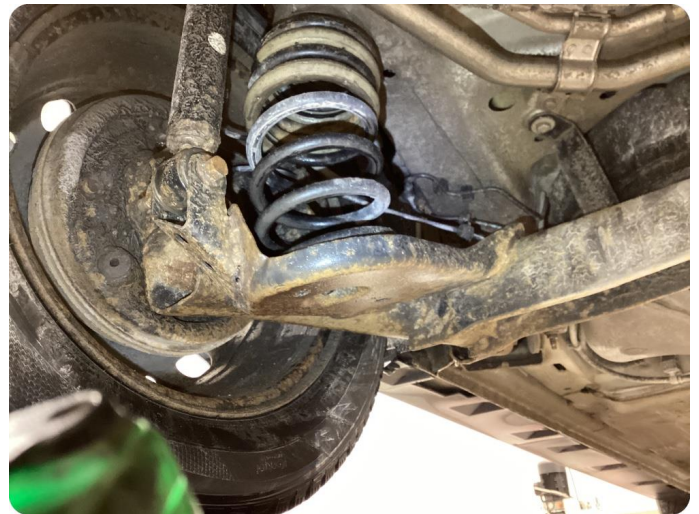
1.2 Rust Anbefaler rust behandling under
