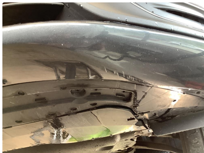
1.2 Noe skrubbskader underkant
