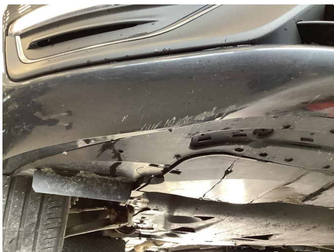
1.2 Noe skrubbskader underkant
