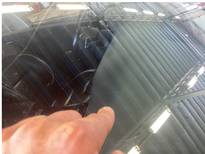
1.5 Steinsprut utenfor synsfelt
