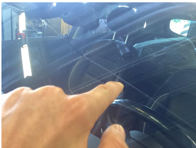
1.5 Steinsprut utenfor synsfelt
