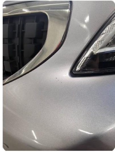
1.7 Steinsprut i front
