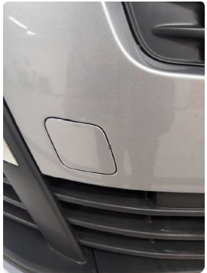
1.7 Steinsprut i front
