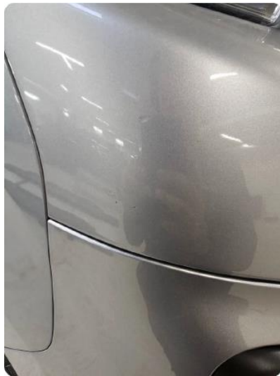
1.7 Steinsprut i front
