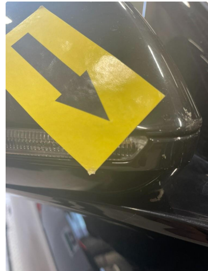
2.1 Krakelering i plast
