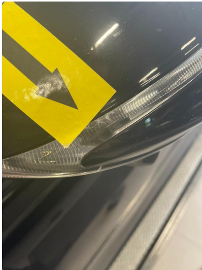
2.1 Krakelering i plast
