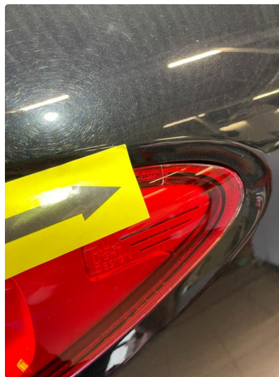
2.2 Defekt / sprukket glass
