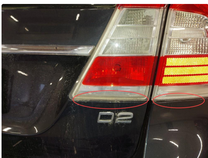
2.1 Krakelering i plast
