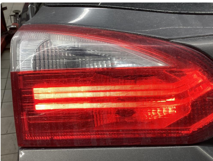
2.2 Krakelering i plast
