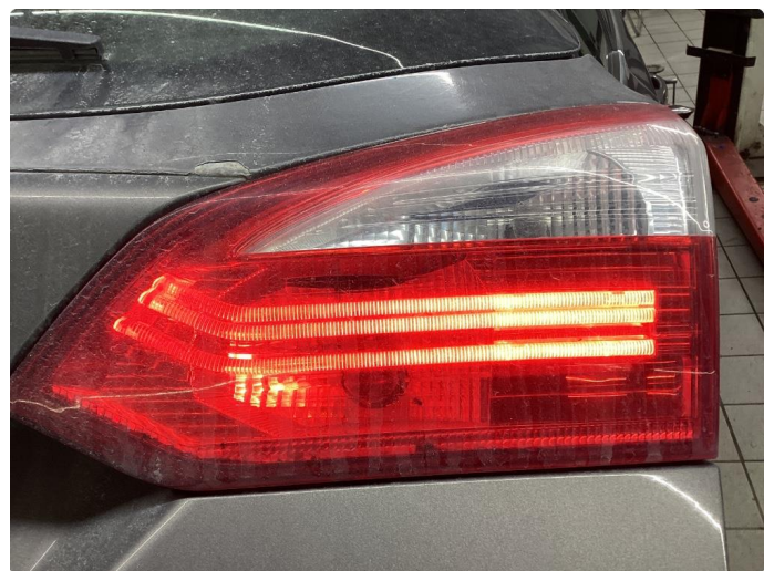
2.2 Krakelering i plast
