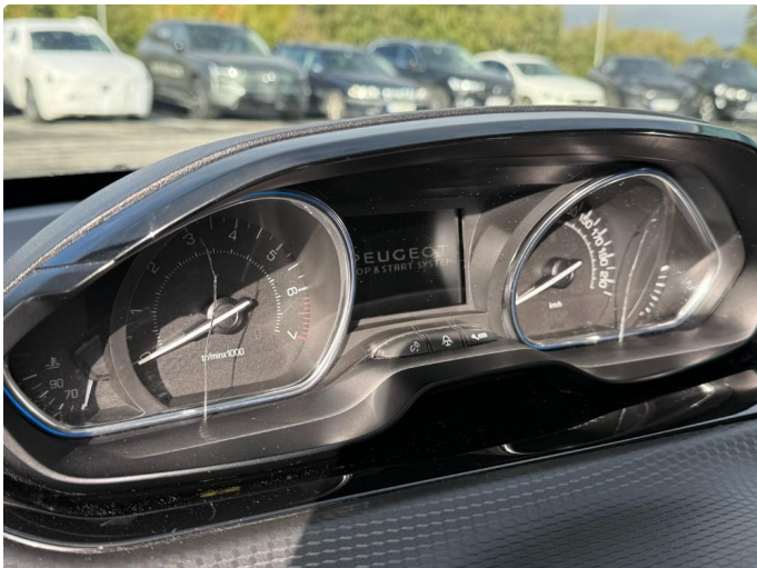
1.1 Sprekker i instrument.
